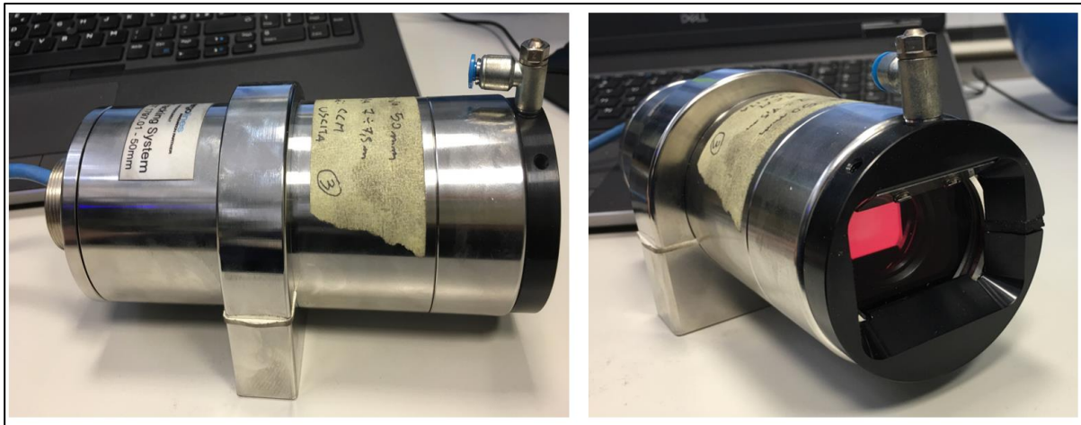
Figure 4: a protection box has been introduced to challenge against dust and partially against heat
