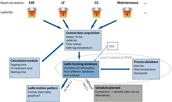
Figure 1: Layout of software tool for ladle tracking
