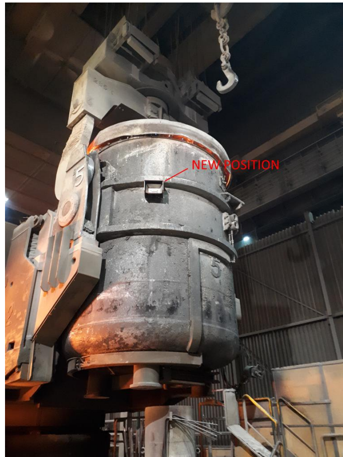
Figure 9: Ladle with SAW tag at new position being inserted in CC waiting position with crane
