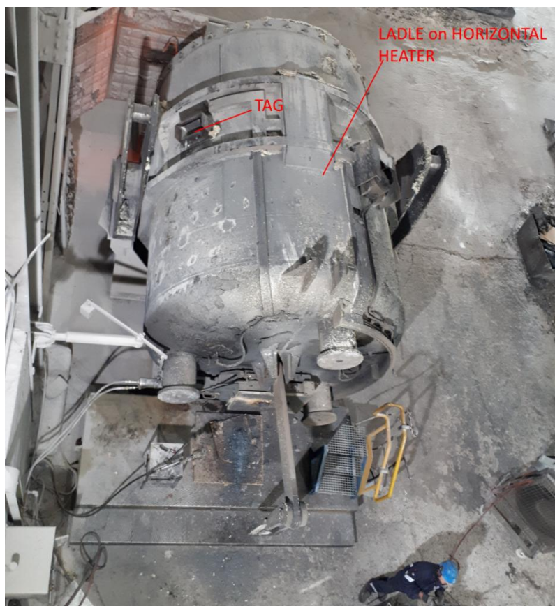
Figure 8: Ladle waiting on horizontal heater – Very hard to place antennas
