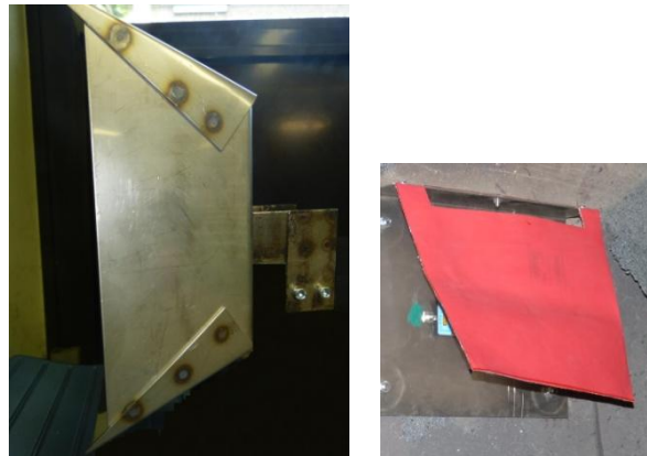
Figure 3: Holder for SAW tag (left) to be mounted to the ladle and exemplary image of mat of insulation material (right)
