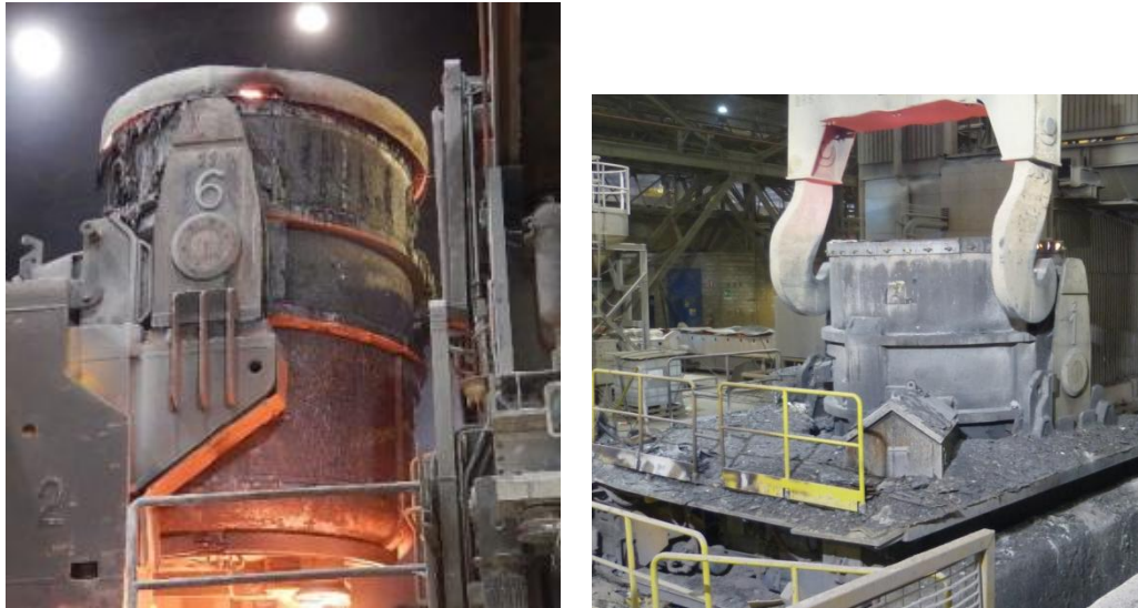
Figure 2: Photographs of ladles in operation, showing splashing in the upper part (left) and ladle inserted in a ladle car (right)
