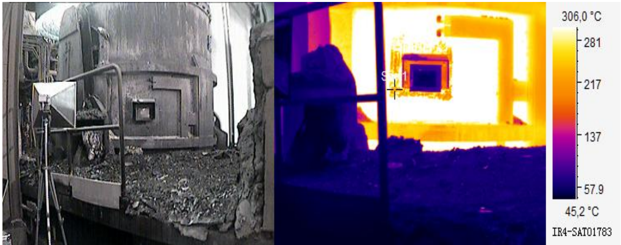
Figure 6: Visual (left) and infrared (right) images of ladle with SAW tag attached
