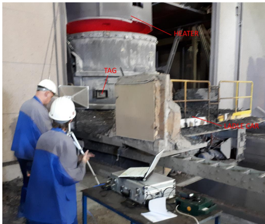
Figure 5: Plant trial using large horn antenna with ladle (equipped with SAW tag) positioned in ladle car under heater
