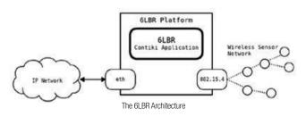
A 6LoWPAN Border Router connects 6LoWPAN devices to the Internet and is responsible for handling traffic to and from its IPv6 and 802.15.4 interfaces. CETIC has developed 6LBR, a deployment-ready solution for border routers, based on the Contiki OS. 6LBR implements mechanisms which complement existing standards to address the issues surrounding the interconnection of IPv6 (NDP) control protocols with RPL, the routing protocol used for IoT sensor networks.
