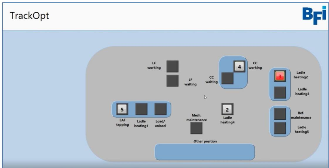
Figure 4: GUI displaying ladles at different stations with ladle mix-up in position "Ladle heating 2"
