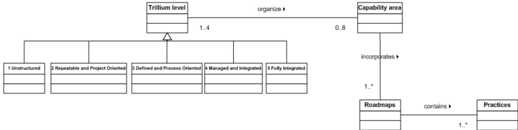
Figure 7 Class Diagram of Trillium 3.0
