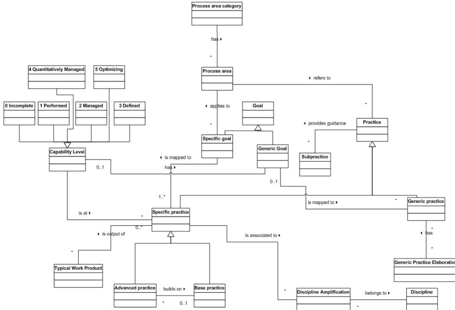
Figure 11 Class Diagram of CMMI 1.1 - Continuous Representation
