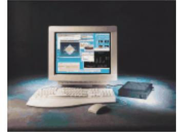
The Unix business architecture, in contrast, relies on smart displays to provide desktop access to centralized Unix servers. These, like the NCD shown above, typically offer large screens, high resolution, fast graphics and extreme reliability. They have no moving parts and no user-accessible operating system. People just turn them on, log in to the machine of their choice and start using applications.
